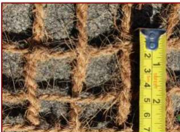
Coir geo-textiles specifications: Grade I- 400g/m 2
